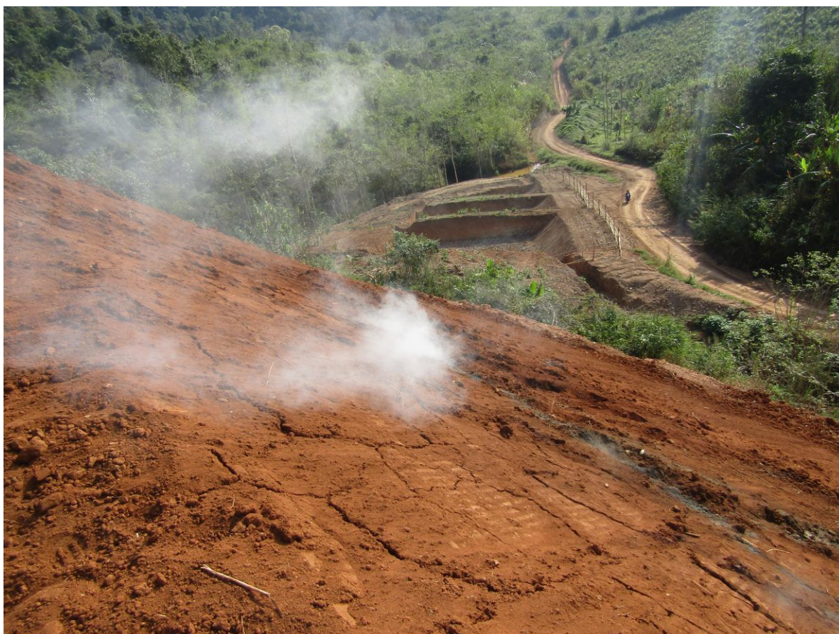
The burning originated by coal own combustion on Ban Chaung coal mine: Photo by Vichai Juntavaro
